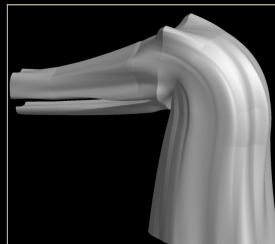
Creature generated by lofting the profiles along the skeleton
